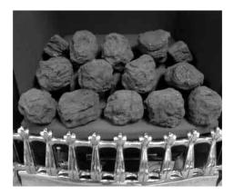
g) Select the remaining four coals and position along the rear edge of the fuelbed (see fig. 7 below)
