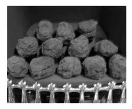
f) Select the two small coals and position to fill the gaps at each end of the third row of coals, as shown. below in Fig. 6
